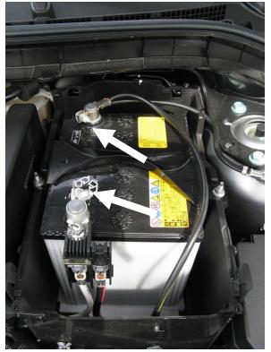
• Using a 10mm socket remove the 3 bolts in the bottom of the battery box shown below.
