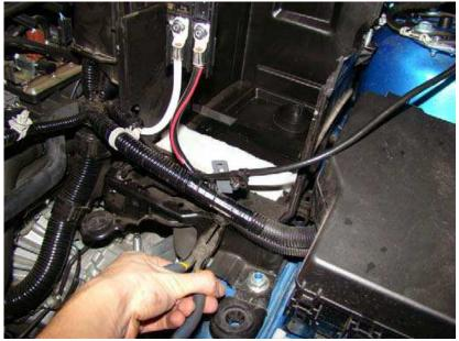
• Using needle nose pliers remove the black connector holding the wiring harness shown below. Tilt the battery box towards the front of the car and remove
