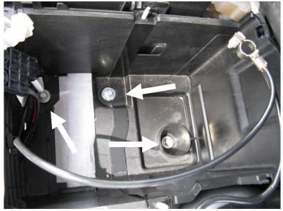
• Using needle nose pliers remove the two grey connectors and 1 black connector securing the wiring to the front side of the battery box shown below.
