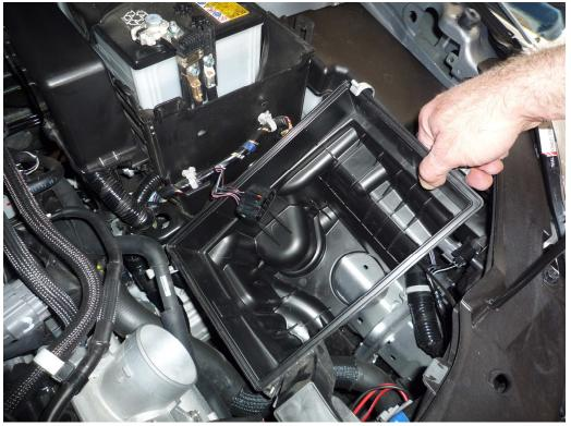
• Using needle nose pliers remove the MAF wire from the back/bottom half of the air box shown below.
