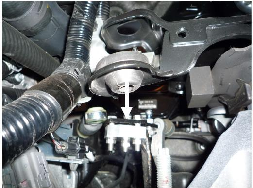
• Re-attach the shifter cable by centering the cable over the new ball stud and pushing down until you here it snap in to place as shown below.
