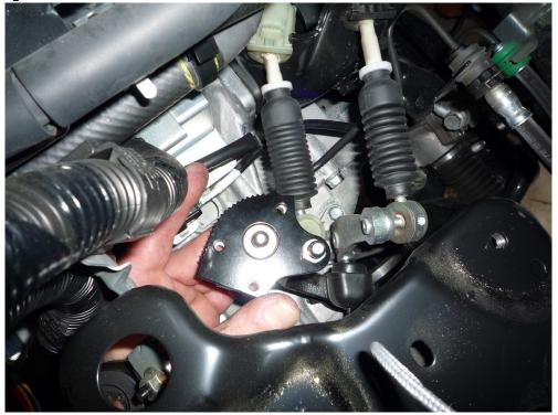
• Install each of the 3 bolts with washers through both the top and bottom half of the shifter plate assembly as shown below.
