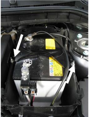
• Using a 10mm socket remove the negative battery cable FIRST then the positive cable and remove the batter from the car shown below.
