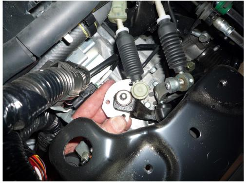
• With your other hand place the top half of the shifter plate on to the shifter arm as shown below.
