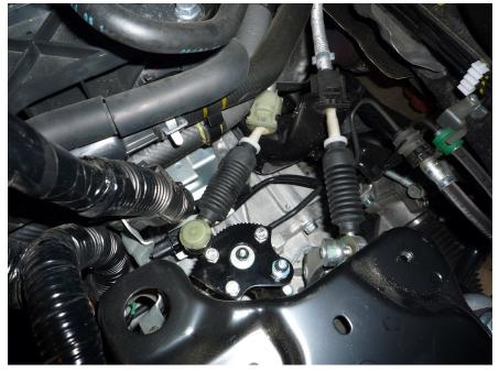
• Put 1 lock washer and 1 nut on each of the 3 assembly bolts and leave them loose. I've added an additional nut and washer to the kit in case you drop or loose one. Now with the bolts snug but not tight, rotate the shift plate assembly slightly clockwise to ensure both ball studs are in line and the assembly is in line with the factory shifter arm as shown below.
