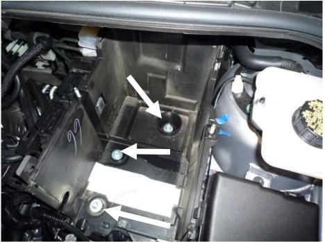
• Remove the hose from the clamp at the back of the battery box shown below. Tilt the battery box towards the front of the vehicle and remove the battery box.
