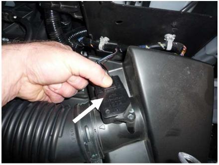
• Remove the rubber hoop holding the bottom half of the air box as shown below.
