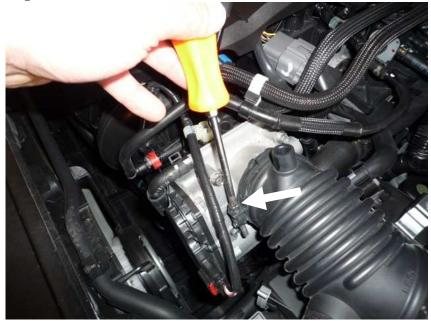
• Unclip all the clips holding the top half of the air filter box to the bottom half as shown below.
