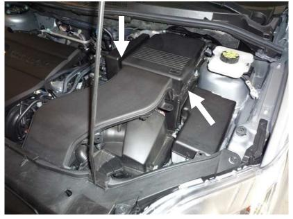
• Remove the battery air scoop by lifting it up out of the front of the battery box and pulling towards the rear of the vehicle and out from the front as shown below.
