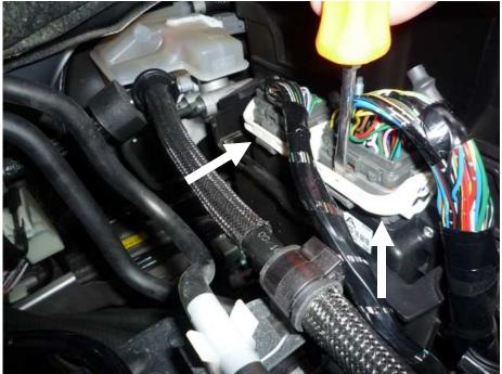
• Slip the wire harness loom out of the hoop shown below.
