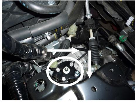
• Using a 10mm wrench and a 10mm socket and socket wrench, tighten the assembly as evenly as possible as shown from a side view below. Do not over tighten the bolts or you WILL strip them and it will be very difficult should you ever need to remove the kit.
