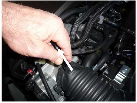
• Loosen the intake hose clamp shown below with a Philips head screw driver.
