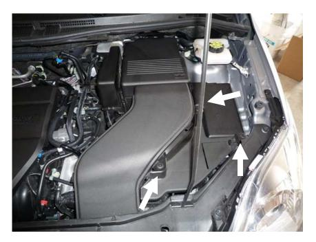
• Spread the 2 tabs on either side of the battery box cover and remove the cover as shown below.
