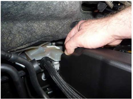
• Using needle nose pliers pinch the connector on the front of the ECU cover and remove the cover as shown below.
