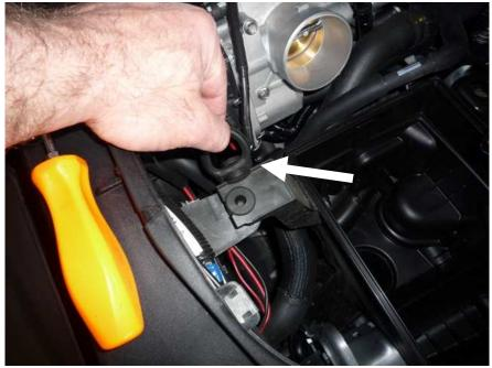
• Tug/Pull up on the bottom half of the air box shown below and remove from the vehicle.
