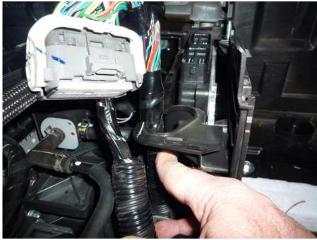
• Using a 12mm socket remove the 3 bolts in the bottom of the battery box shown below.
