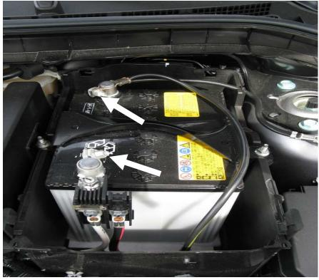
• Using needle nose pliers remove the black wire connector from the front cover of the battery box as shown below.
