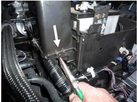
• Using a 10mm socket and socket wrench remove the nuts holding the cross bar over the top of the battery and remove the cross bar.
