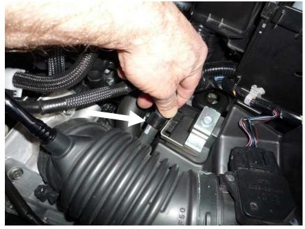
• Remove the tube shown below by pulling it out of the intake hose.
