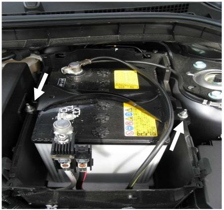
• Using a 10mm socket remove the negative battery cable FIRST then the positive cable and remove the batter from the car shown below.
