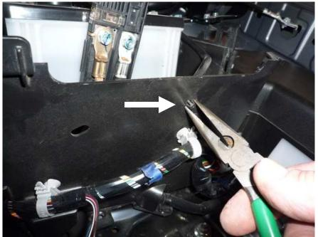
• With front cover of the battery box laying forward remove the 2 grey wire connectors as shown below and remove the cover from the vehicle.
