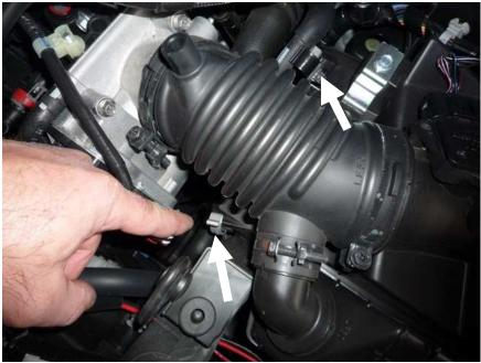
• Remove the connector for the MAF sensor shown below. Then remove the whole top section of the intake and air box from the vehicle.
