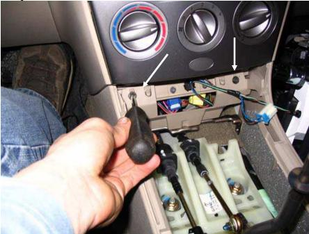
Now remove the 4x12mm bolts located at each corner of the shifter cage. Raise the cage up to clear the studs. Pry the steel sleeves up and out of the rubber grommets.
