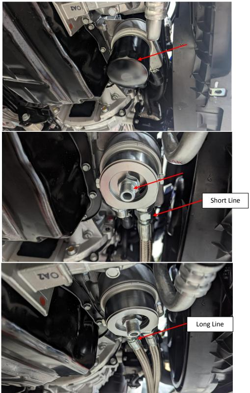
14. Reinstall the oil filter and wrap each line with the heat shields provided in your kit. Be sure you have no oil on your hands when doing this or the adhesive will not stick. Add one 8" zip tie where shown below.
