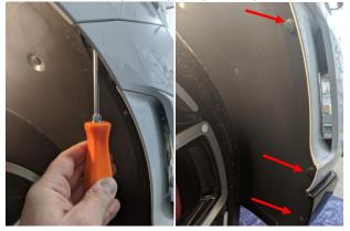
3. Using your hands pull the bumper cover away from the fender starting at the end closest to the wheel well. Repeat on both sides.
