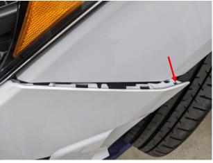
4. Using a 10mm socket, remove the 10, 10mm bolts in the next series of pictures.
