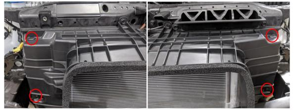
10. Using 3, 6mm bolts, 6 flat washers, and 3 nuts, mount the upper mounting bracket to the top of the cowl. Admittedly, this is a pain in the ass but doable. Supporting the oil cooler core on the box your kit shipped in, will make this easier.
