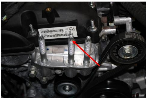
9. Install your new JBR Passenger mount in the vehicle. You may need to raise the motor a bit more. Some wiggling of the motor may be necessary to fit the mount. Place a lock washer then a flat washer on to each of the bolts included with the mount. Loosely install all three and then tighten all three 19mm bolts to 45ft/lbs.
