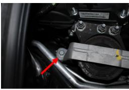
8. Remove the mount from the car. Using a E10 torx socket remove the three studs from the motor.
