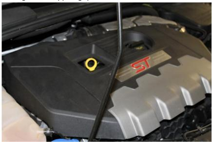
4. Remove the coolant reservoir by pulling it straight up, then rotating it and laying over on the the top of the engine being careful not to kink the lines attached to it
