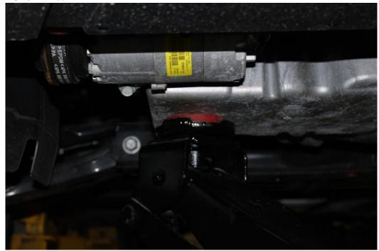
6. Remove the three 19mm nuts securing the top portion of the OEM motor mount to the engine.
