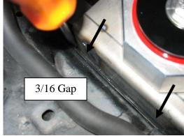
12. Re-install the coolant and/or power steering reservoirs.
