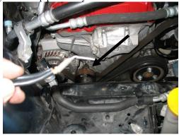
9. Flatten the tab on the end of the ground strap previously bolted to the chassis.
