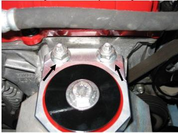
11. Next install the two 17mm bolts and tighten to 70 Foot-pounds. Moving the motor may be required for the holes in the chassis to line up with the holes in the mount. Ensure there is approximately a 3/16" gap between the chassis and the back of the motor mount. A flat head screw driver may be used to move the mount in to place while tightening. Never attempt to loosen the bushing bolt, doing so will void the warranty on the mount.
