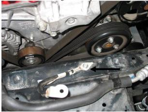
8. Bend the end of the ground strap previously bolted to the mount on a 45\* angle.
