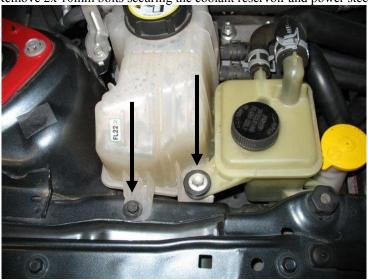
5. (All Years) Remove the coolant and power steering reservoirs by inserting a flat head screw driver in to the tabs and pulling up.
