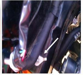
10. Place your new JBR Passenger Motor Mount in place and tighten to 60 Foot-pounds.
