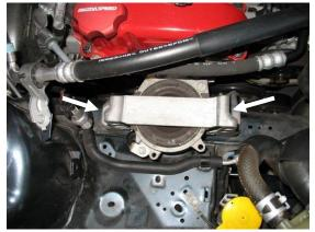
7. Remove 1x 10mm bolt and remove the ground strap.
