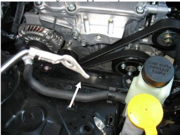
9. Remove the 8mm timing cover bolt located towards the rear of the vehicle above the alternator. Attach the end of the ground strap previously attached to the factory mount that you bent on a 45\* degree angle in step 7 and tighten. Attach the other end of the ground strap using the 10mm bolt removed in step 6 to the rear most pre-existing hole in the sub-frame located in front of the alternator.
